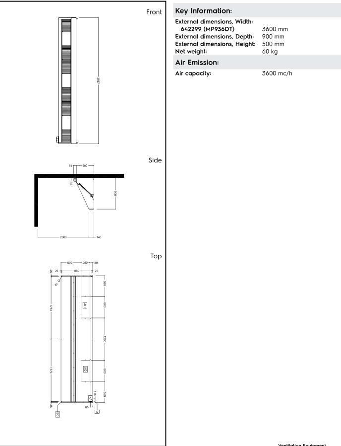
Ventilation Equipment 304 S/S Wall Hood+Filters 3600X900mm
